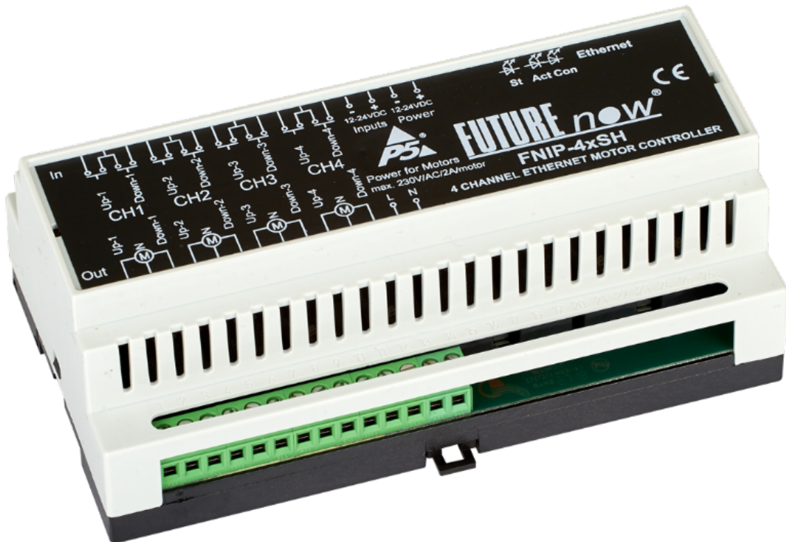
The FNIP-4xSH Window Shading Controller
